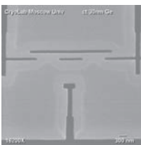
Fig. 3. SEM image of the structure. Dark places correspond to holes, while light colors correspond to absence of copolymer. Sample: E-beam lithography mask for fabrication SET devices by shadow evaporation technique. V. A. Krupenin, Cryoelectronics Lab., Physical department of MSU, Moscow, Russia.
