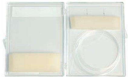
Box with MF012 SNOM probes
